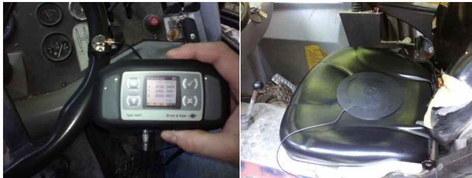
Figure 1 : a. Measuring of vibrations on the steering wheel b. Measuring of vibrations on the seat
